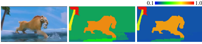
Fig. 3. Significance map generation. Left: input video frame; middle: significance map; right: enhanced significance map. Significance values are visualized by colors ranging from blue (lowest significance) to red (highest significance).
